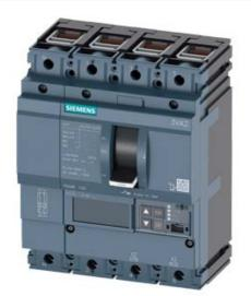
CIRCUIT BREAKER 3VA2 IEC FRAME 100 BREAKING CAPACITY CLASS H ICU=85KA @ 415 V 4POLE, LINE PROTECTION ETU550, LSI, IN=63A OVERLOAD PROTECTION IR=25A ...63A SHORT CIRCUIT PROTECTION ISD=0,6..10X IN, II=1,5..12X IN NEUTRAL PROTECTION ADJUSTABLE (OFF, UPTO 160%) CABLE CONNECTION
