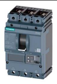
CIRCUIT BREAKER 3VA2 IEC FRAME 160 BREAKING CAPACITY CLASS C ICU=110KA @ 415 V 3POLE, LINE PROTECTION ETU560, LSIG, IN=100A OVERLOAD PROTECTION IR=40A ...100A SHORT CIRCUIT PROTECTION ISD=0,6..10X IN, II=1,5..12X IN NEUTRAL PROTECTION OPTIONAL WITH EXT. CT,UPTO 160% GROUNDFAULT, SWITCHABLE IG=0,2... 1 X IN, TG=0,050,8MS BUSBAR CONNECTION
