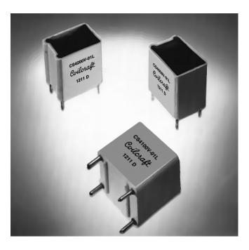
These low cost Coilcraft current sensing transformers are designed for use up to 100 kHz. They incorporate the current and sense windings in one small, encapsulated package requiring minimum board space.
