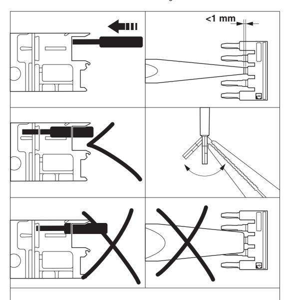
Please note a reduction of the nominal voltage if the FBS bridges are configured by breaking out contact tabs or cutting to a specific length
