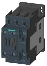
CONTACTOR, AC-3, 11KW/400V, 1NO+1NC, AC 200V 50HZ, 200...220V 60HZ, 3-POLE, SZ S0 SCREW TERMINAL
