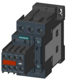
CONTACTOR, AC-3, 18.5KW/400V, 2NO+2NC, DC 24V, 3-POLE, SZ S0 SCREW TERMINAL PERMANENT AUX. SWITCH FOR SUVA APPLICATIONS
