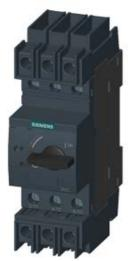
CIRCUIT-BREAKER SZ S00, FOR PLANT PROTECTION, WITH APPROBATION CIRCUIT-BREAKER UL 489. CSA C22.2 NO.5-02. A-RELEASE 2 A, N-RELEASE 26 A, SCREW CONNECTION, STANDARD SW. CAPACITY
