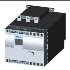
SIRIUS SOFT STARTER, VALUES WITH 575 V, 50 DEG., STANDARD: 145A, 125HP, INSIDE-DELTA CIRCUIT 3: 251A, 250HP, 400-690 V AC, 115 V AC, CAGE CLAMP TERMINALS
