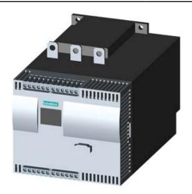
SIRIUS SOFT STARTER, VALUES WITH 690 V, 40 DEG., STANDARD: 162A, 160KW, INSIDE-DELTA CIRCUIT 3: ONLY UP TO 600V, 400-690 V AC, 230 V AC, SCREW TERMINALS
