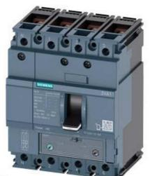
CIRCUIT BREAKER 3VA1 IEC FRAME 160 BREAKING CAPACITY CLASS N ICU=25KA @ 415 V 4-POLE, LINE PROTECTION TM240, ATAM, IN=50A OVERLOAD PROTECTION IR=35A ...50A SHORT CIRCUIT PROTECTION II=5...10 X IN NEUTRAL UNPROTECTED BUSBAR CONNECTION
