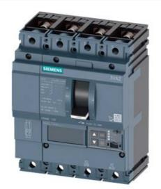
CIRCUIT BREAKER 3VA2 IEC FRAME 100 BREAKING CAPACITY CLASS H ICU=85KA @ 415 V 4POLE, LINE PROTECTION ETU550, LSI, IN=100A OVERLOAD PROTECTION IR=40A ...100A SHORT CIRCUIT PROTECTION ISD=0,6..10X IN, II=1,5..12X IN NEUTRAL PROTECTION ADJUSTABLE (OFF, UPTO 100%) BUSBAR CONNECTION
