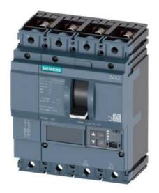
CIRCUIT BREAKER 3VA2 IEC FRAME 160 BREAKING CAPACITY CLASS M ICU=55KA @ 415 V 4POLE, LINE PROTECTION ETU550, LSI, IN=160A OVERLOAD PROTECTION IR=64A ...160A SHORT CIRCUIT PROTECTION ISD=0,6..10X IN, II=1,5..10X IN NEUTRAL PROTECTION ADJUSTABLE (OFF, UPTO 100%) BUSBAR CONNECTION
