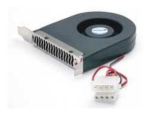
The StarTech.com PC case exhaust fan is an add-in cooling fan designed to fit in the PCI or ISA expansion slots of any computer. It is used to exhaust warm air out, preventing problems due to overheating components. The exhaust fan inlet faces adjacent PCI or AGP cards and makes a great video card cooler for hot running 3D accelerator cards like the Voodoo, TNT2, GeForce256 and others. Power is supplied to the fan using a standard LP4 (hard drive power connector) pass through plug.
