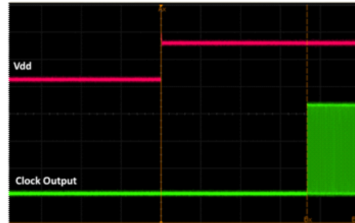
Figure 16. Startup Waveform vs. Vdd
