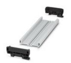
Profile housing (PA), mounting type: DIN rail mounting, color: light gray (7035), dimensions on the DIN rail: width: 253.8 mm, height: 92.3 mm, depth: 39.45 mm, incl. 2 lateral elements (PA), color: black (9005), for PCBs with width: 72 mm, length: 250 mm, PCB surface: 15780 mm²
