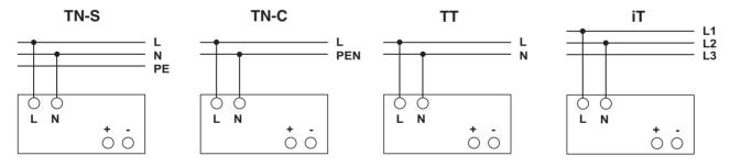
The 100 V AC  $\dots$  240 V AC connection is made using the L and N screw connections.
