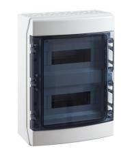
The IP65 boxes have a completely new and innovative shape, reaching the highest level of quality and design. They are made from halogen free long-lasting thermoplastic materials, ABS and polycarbonate. They have lots of space for wiring and also the possibility to place the Din rail in two height positions. Mounting plates and other accessories can be installed on the base inside.
