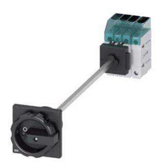
Switch disconnector 3LD3, main switch 3-polig + N, lu 16A operational switch at AC-23 A at 400 V 7,5 kW floor mounting Base mounting with door coupling center-hole 22,5 mm rotary operationg mechanism black  $66 \times 66$  mm
