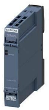
Thermistor motor prot. relay Compact evaluation unit 17.5 mm enclosure Spring-type terminals 1 CO contact US = 24 V-240 V AC/DC Auto RESET Suitable for bimetal switches Supply = output voltage 1 LED (READY)
