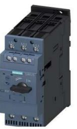
CIRCUIT BREAKER, SIZE S2, FOR MOTOR PROTECTION, CLASS 10, A-RELEASE 42...52A, N-RELEASE 741A, SCREW TERMINAL, STANDARD BREAKING CAPACITY W. TRANSV. AUX. SWITCH 1NO+1NC
