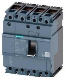
CIRCUIT BREAKER 3VA1 IEC FRAME 160 BREAKING CAPACITY CLASS S ICU=36KA @ 415 V 4-POLE, LINE PROTECTION TM210, FTFM, IN=16A OVERLOAD PROTECTION IR=16A FIXED SHORT CIRCUIT PROTECTION II=10 X IN NEUTRAL UNPROTECTED BUSBAR CONNECTION
