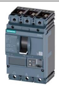
CIRCUIT BREAKER 3VA2 IEC FRAME 100 BREAKING CAPACITY CLASS C ICU=110KA @ 415 V 3POLE, LINE PROTECTION ETU860, LSIG, IN=63A OVERLOAD PROTECTION IR=25A ...63A SHORT CIRCUIT PROTECTION ISD=0,6..10X IN, II=1,5..12X IN NEUTRAL PROTECTION OPTIONAL WITH EXT. CT,UPTO 160% GROUNDFAULT, SWITCHABLE IG=0,2... 1 X IN, TG=0,050,8MS BUSBAR CONNECTION
