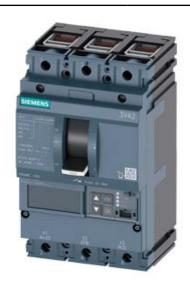
CIRCUIT BREAKER 3VA2 IEC FRAME 160 BREAKING CAPACITY CLASS M ICU=55KA @ 415 V 3POLE, LINE PROTECTION ETU560, LSIG, IN=63A OVERLOAD PROTECTION IR=25A ...63A SHORT CIRCUIT PROTECTION ISD=0,6..10X IN, II=1,5...12X IN NEUTRAL PROTECTION OPTIONAL WITH EXT. CT,UPTO 160% GROUNDFAULT, SWITCHABLE IG=0,2... 1 X IN, TG=0,050,8MS CABLE CONNECTION
