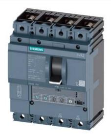
CIRCUIT BREAKER 3VA2 IEC FRAME 250 BREAKING CAPACITY CLASS L ICU=150KA @ 415 V 4POLE, LINE PROTECTION ETU350, LSI, IN=160A OVERLOAD PROTECTION IR=64A ...160A SHORT CIRCUIT PROTECTION ISD=1,5... 10 X IR, II=12 X IN NEUTRAL PROTECTION ADJUSTABLE(OFF,50%,100%) BUSBAR CONNECTION
