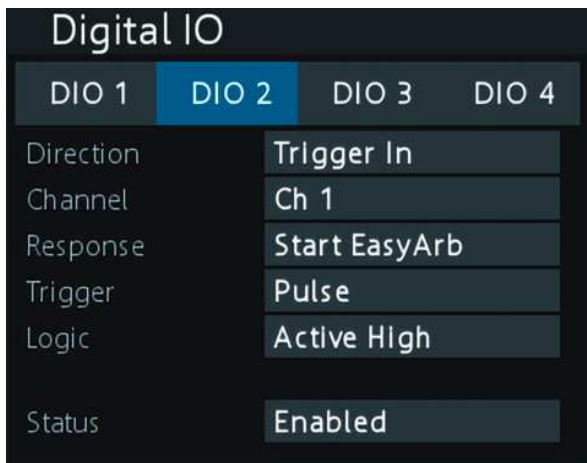
Here, channel 1 of the optional digital I/O interface (R&S®NGE-K103) is used as a trigger input
