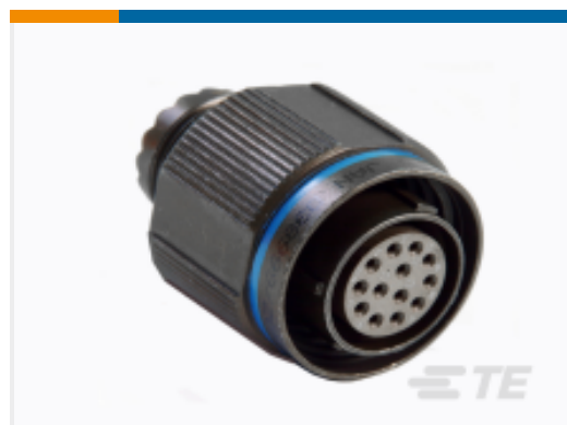
TE Part #YDTS26G21-39SNV001 D38999: Straight Plug, 21-39 Insert
