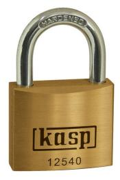
~ Hardened steel shackle ~ Double bolted locking mechanism ~ Solid brass body ~ Anti pick mushroom pins ~ Paracentric keyway ~ Supplied with 2 keys ~ Keyed alike, all padlocks of this order code can be opened with the same key ~ Padlock width: 40 mm ~ Shackle diameter: 6,4 mm ~ Internal shackle height: 22 mm
