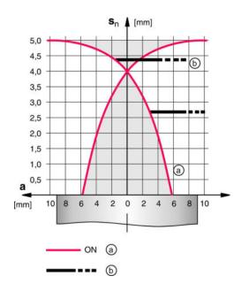
a Inductive switchb Standard measuring plate
