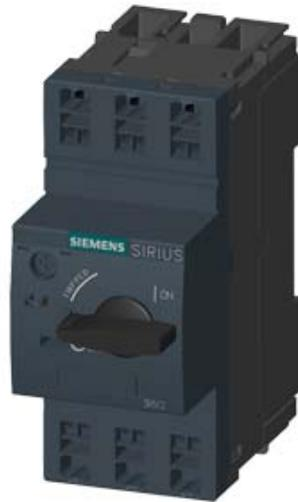
LEISTUNGSSCHALTER BGR. S00, FUER DEN TRAFOSCHUTZ A-AUSL.0,45...0,63A, N-AUSL.13A FEDERZUGANSCHLUSS, STANDARDSCHALTVERMOEGEN
