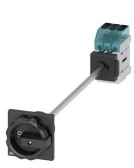
Switch disconnector 3LD3, main switch 3-polig, lu 63A operational switch at AC-23 A at 400 V 22,0 kW floor mounting Base mounting with door coupling center-hole 22,5 mm rotary operationg mechanism black 66 x66 mm
