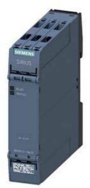
Thermistor motor prot. relay Standard evaluation unit 22.5 mm enclosure Screw terminals 2 CO contacts US = 24 V AC/DC Auto RESET Suitable for bimetal switches 2 LEDs (READY/TRIPPED) Galvanic separation
