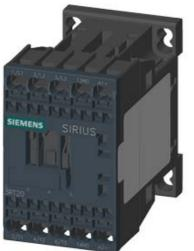
COUPLING RELAY, AC-3, 3KW/400V, 1NO, DC 24V, 0.7...1.25\*US, W. INTEGR. SUPPRESSORDIODE, SZ S00, SPRING-LOADED TERMINAL
