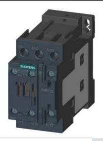
CONTACTOR, AC-3, 5.5KW/400V, 1NO+1NC, DC 220V, 3-POLE, SZ S0 SCREW TERMINAL
