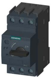
SPECIAL TYPE CIRCUIT BREAKER SIZE S00, FOR MOTOR PROTECTION, CLASS 10, A-RELEASE 2.8...4A, SHORT-CIRCUIT RELEASE 52A, SCREW TERMINAL, STANDARD SWITCHING CAPACITY AMBIENT TEMPERATURE -50 DEGREES C 500 SWITCHING CYCLES
