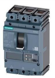
CIRCUIT BREAKER 3VA2 IEC FRAME 100 BREAKING CAPACITY CLASS L ICU=150KA @ 415 V 3POLE, LINE PROTECTION ETU560, LSIG, IN=63A OVERLOAD PROTECTION IR=25A ...63A SHORT CIRCUIT PROTECTION ISD=0,6..10X IN, II=1,5..12X IN NEUTRAL PROTECTION OPTIONAL WITH EXT. CT,UPTO 160% GROUNDFAULT, SWITCHABLE IG=0,2... 1 X IN, TG=0,050,8MS CABLE CONNECTION
