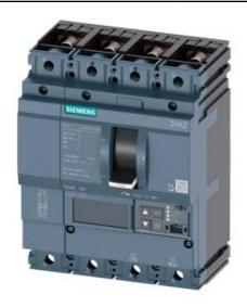
CIRCUIT BREAKER 3VA2 IEC FRAME 160 BREAKING CAPACITY CLASS C ICU=110KA @ 415 V 4POLE, LINE PROTECTION ETU560, LSIG, IN=63A OVERLOAD PROTECTION IR=25A ...63A SHORT CIRCUIT PROTECTION ISD=0,6..10X IN, II=1,5..12X IN NEUTRAL PROTECTION ADJUSTABLE (OFF, UPTO 160%) GROUNDFAULT, SWITCHABLE IG=0,2... 1 X IN, TG=0,050,8MS BUSBAR CONNECTION
