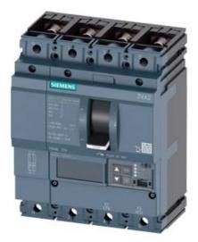
CIRCUIT BREAKER 3VA2 IEC FRAME 250 BREAKING CAPACITY CLASS H ICU=85KA @ 415 V 4POLE, LINE PROTECTION ETU850, LSI, IN=250A OVERLOAD PROTECTION IR=100A ...250A SHORT CIRCUIT PROTECTION ISD=0,6..10X IN, II=1,5..10X IN NEUTRAL PROTECTION ADJUSTABLE (OFF, UPTO 100%) BUSBAR CONNECTION
