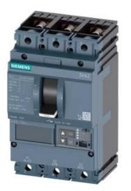
CIRCUIT BREAKER 3VA2 IEC FRAME 250 BREAKING CAPACITY CLASS C ICU=110KA @ 415 V 3POLE, LINE PROTECTION ETU560, LSIG, IN=250A OVERLOAD PROTECTION IR=100A ...250A SHORT CIRCUIT PROTECTION ISD=0,6..10X IN, II=1,5..10X IN NEUTRAL PROTECTION OPTIONAL WITH EXT. CT,UPTO 160% GROUNDFAULT, SWITCHABLE IG=0,2... 1 X IN, TG=0,050,8MS BUSBAR CONNECTION
