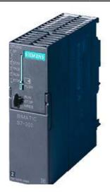
SIMATIC S7-300, CPU 312 CPU WITH MPI INTERFACE, INTEGRATED 24 V DC POWER SUPPLY 32 KBYTE WORKING MEMORY, MICRO MEMORY CARD NECESSARY
