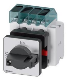
Switch disconnector 3LD3, main switch 3-polig + N, lu 16A operational switch at AC-23 A at 400 V 7,5 kW front mounted Base mounting with center-hole 22,5 mm knob-operated mechanism black  $48 \times 48$  mm with auxiliary 1NO+1NC
