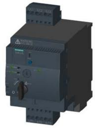
SIRIUS, COMPACT STARTER, REVERSING STARTER 690 V, 24 V AC/DC, 50 ... 60 HZ, 0.1 ... 0.4 A, IP20, MAIN CIRCUIT CONNECTION: SPRING-LOADED TERMINAL, AUXILIARY CIRCUIT CONNECTION: PLUG-IN, W/O TERMINALS
