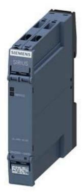
Thermistor motor prot. relay Compact evaluation unit 17.5 mm enclosure Screw terminals 1 CO contact US = 24 V-240 V AC/DC Auto RESET Suitable for bimetal switches Supply = output voltage 1 LED (READY)
