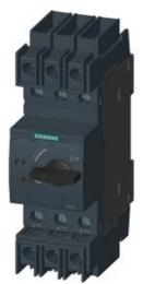
CIRCUIT-BREAKER SZ S00, FOR TRANSFORMER PROTECTION, WITH APPROBATION CIRCUIT-BREAKER UL 489. CSA C22.2 NO.5-02. A-RELEASE 1 A, N-RELEASE 21 A, SCREW CONNECTION, STANDARD SW. CAPACITY
