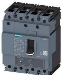
CIRCUIT BREAKER 3VA1 IEC FRAME 160 BREAKING CAPACITY CLASS M ICU=55KA @ 415 V 4-POLE, LINE PROTECTION TM220, ATFM, IN=125A OVERLOAD PROTECTION IR=87,5A ...125A SHORT CIRCUIT PROTECTION II=10 X IN NEUTRAL PROTECTION 100% BUSBAR CONNECTION
