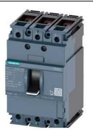
CIRCUIT BREAKER 3VA1 IEC FRAME 160 BREAKING CAPACITY CLASS H ICU=70KA @ 415 V 3-POLE, LINE PROTECTION TM210, FTFM, IN=32A OVERLOAD PROTECTION IR=32A FIXED SHORT CIRCUIT PROTECTION II=10 X IN BUSBAR CONNECTION
