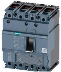
CIRCUIT BREAKER 3VA1 IEC FRAME 160 BREAKING CAPACITY CLASS H ICU=70KA @ 415 V 4-POLE, LINE PROTECTION TM240, ATAM, IN=40A OVERLOAD PROTECTION IR=28A ...40A SHORT CIRCUIT PROTECTION II=5 X IN NEUTRAL PROTECTION 100% BUSBAR CONNECTION
