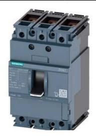
CIRCUIT BREAKER 3VA1 IEC FRAME 160 BREAKING CAPACITY CLASS H ICU=70KA @ 415 V 3-POLE, LINE PROTECTION TM210, FTFM, IN=16A OVERLOAD PROTECTION IR=16A FIXED SHORT CIRCUIT PROTECTION II=10 X IN BUSBAR CONNECTION
