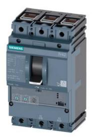
CIRCUIT BREAKER 3VA2 IEC FRAME 100 BREAKING CAPACITY CLASS C ICU=110KA @ 415 V 3POLE, LINE PROTECTION ETU320, LI, IN=25A OVERLOAD PROTECTION IR=10A ...25A SHORT CIRCUIT PROTECTION II=12 X IN CABLE CONNECTION
