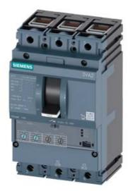
CIRCUIT BREAKER 3VA2 IEC FRAME 160 BREAKING CAPACITY CLASS L ICU=150KA @ 415 V 3POLE, LINE PROTECTION ETU330, LIG, IN=25A OVERLOAD PROTECTION IR=10A ...25A SHORT CIRCUIT PROTECTION II=1,5...12 X IN GROUNDFAULTPROTECTION IG=0,2... 1 X IN, TG=0,1/0,3MS CABLE CONNECTION
