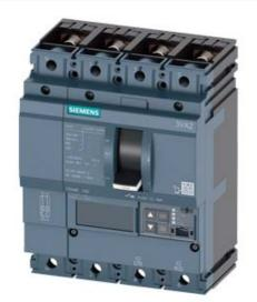
CIRCUIT BREAKER 3VA2 IEC FRAME 160 BREAKING CAPACITY CLASS H ICU=85KA @ 415 V 4POLE, LINE PROTECTION ETU560, LSIG, IN=63A OVERLOAD PROTECTION IR=25A ...63A SHORT CIRCUIT PROTECTION ISD=0,6..10X IN, II=1,5..12X IN NEUTRAL PROTECTION ADJUSTABLE (OFF, UPTO 160%) GROUNDFAULT, SWITCHABLE IG=0,2... 1 X IN, TG=0,050,8MS BUSBAR CONNECTION
